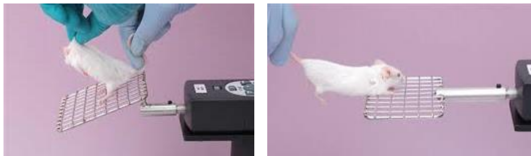
Figure 3.6. Illustration of a grip strength experiment. The rodent was delicately placed on a grid bar that allowed all limbs grasp. The black arrow indicates the direction of the pulling force (adopted from the Internet).
