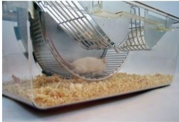
Figure 3.7. Voluntary wheel apparatus (image adopted from https://www.bioseb.com ).
